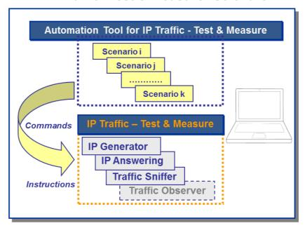
The Automation Tool for "IP Traffic—Test & Measure" software allows editing and executing scenarios to control and set parameters of the "IP Traffic - Test & Measure" software on the same
