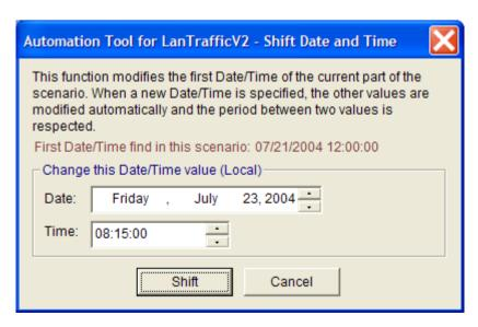
You can define for example a new date & time: 07/23/2004 08:15:00 and then press the 'Shift' button. So, the first command or instruction of the scenario with a date/time will refer to this new value, and automatically all other commands and instructions with a date/time will be updated with this new basis.
