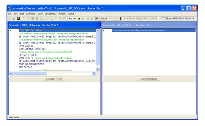
You can switch to the 'Edit Mode' by pressing the 'Edit Mode' button in the Tool Bar.
