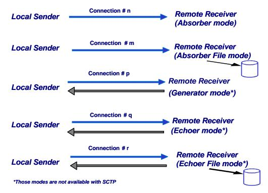
Note: We consider that the local machine is used for sending traffic and the remote one is used for receiving traffic.
