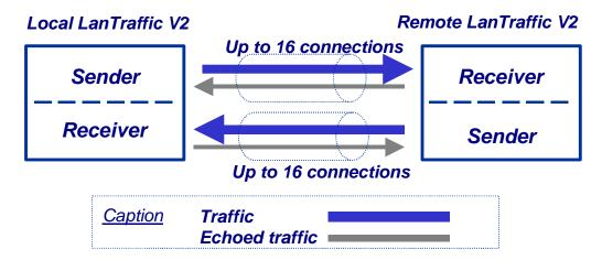
□ The **Sender** generates up to 16 simultaneous UDP (Unicast, Multicast or Broadcast) and/or TCP connections and/or ICMP connections. The connections can be established in two different testing modes:
