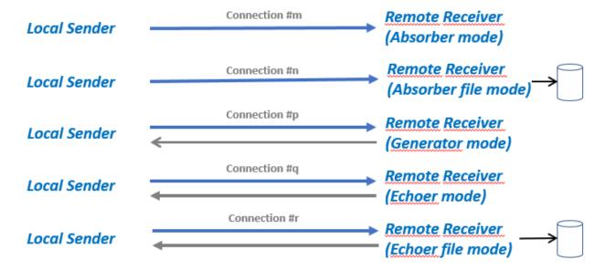
Note: We consider that the local machine is used for sending traffic and the remote one is used for receiving traffic.
