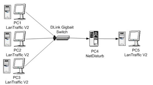
**LanTraffic V2** Unitary Testing Mode is selected and the default values (menu File/new) are kept except for these particular values listed hereafter. Different UDP data sizes are used to realize these tests.
